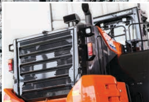
New rear grill protects radiator compartment.
