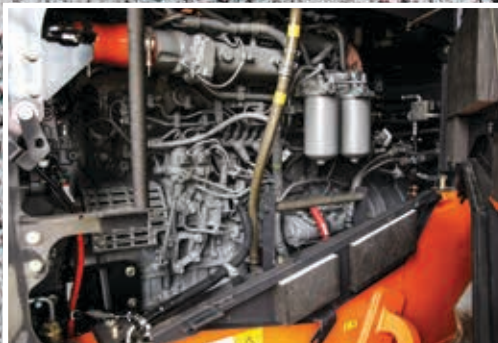
Stage IV engine reduces fuel consumption.
