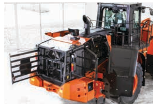
Easy access to the engine compartment.
